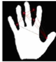
The resulting data capture by a Charge-Coupled Device (CCD) camera of the top view of the hand including example distance measurements.
