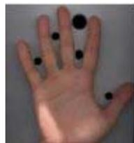
The hand of the subject is placed on the plate, palm down, and guided by five pegs that sense when the hand is in place.
